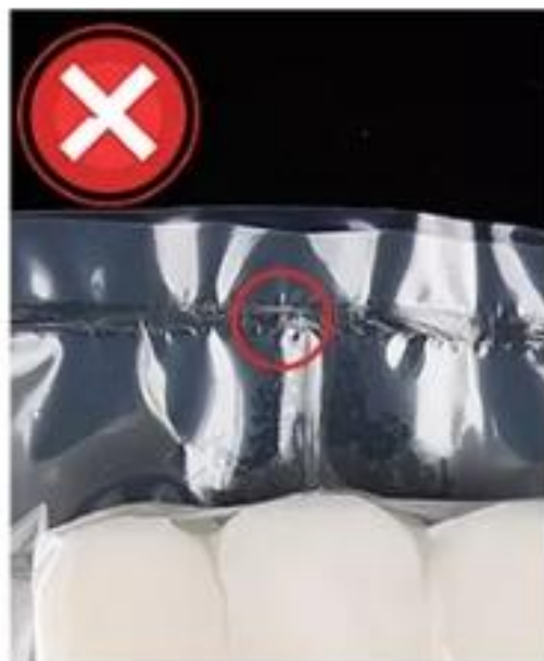
Folded Sealing Leak Easily
