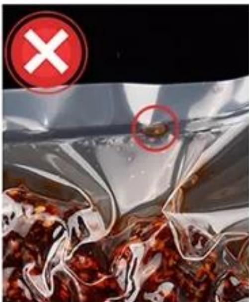
Untidy Sealing Leak Easily
