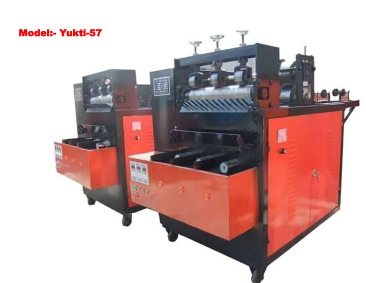
Capacity:- 15kg/hour for spiral round scrubber and 14kg/hour for flat scrubber. Warranty:- one year. Service:- online. Wire Diameter:- 0.13mm. Voltage:- 220v/380v. Scrubber size:- 10g to 50g. Operation:- One person. Control System:- Frequency conversion.
