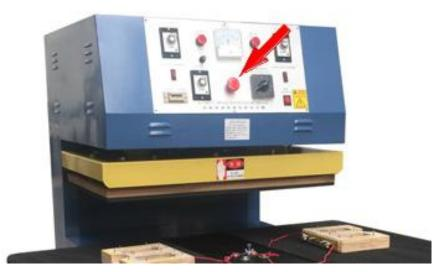
Emergency stop button Install the emergency stop button, can stop working anytime, ensure the safety of operator also reduce the output of defective products.
