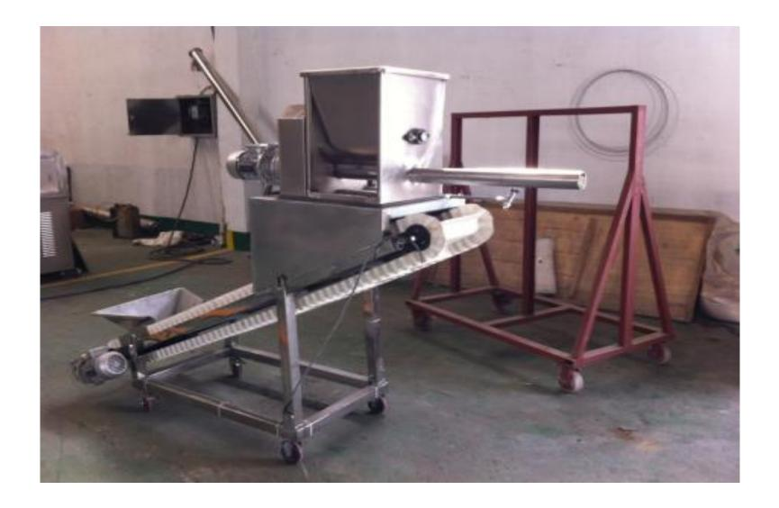
Installed Power: 1.12kw Power consumption: 1kw Capacity: 100-250kg/h Dimension: 1600×600×1700mm
