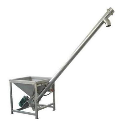
Installed capacity: 1.1kw 380v/50hz Power consumption: 0.5kw Dimensions mm: 3100 \* 590 \* 2200mm
