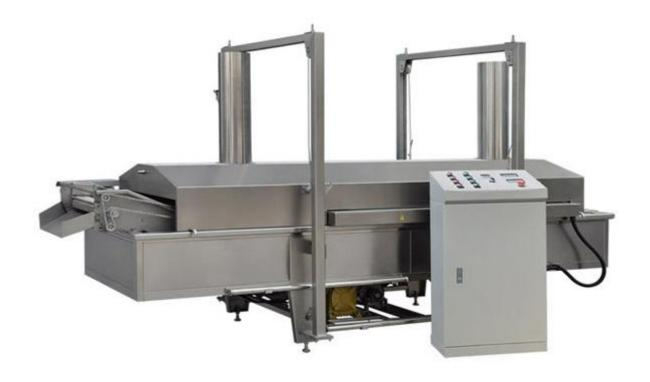
Dimension: 2500\*700\*2100mm height can be adjusted Oil groove size: 2000\*500\*400mm (length\*width\*depth) Mesh belt width: 500mm Oil capacity: 400L Installed power: 48KW Transmission
