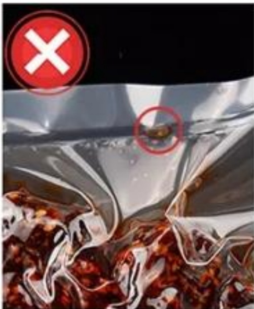
Untidy Sealing Leak Easily
