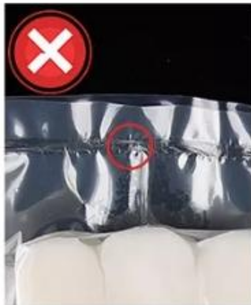
Folded Sealing Leak Easily
