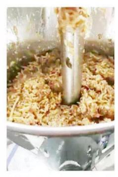
3.Put the prepared filling into the filling hopper of the machine.
