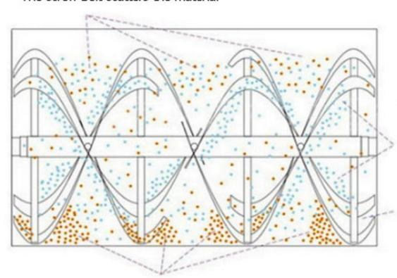
The inner spiral belt sends the inner material to both sides
